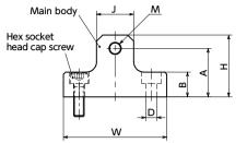
\*: Check the A dimension based on the distance from the mounting surface to the top surface of the table and select accordingly.
