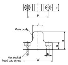
\*: Check the H dimension based on the distance from the mounting surface to the top surface of the table and select accordingly.
