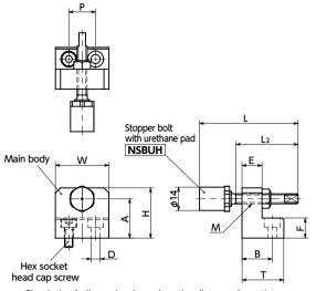
\*: Check the A dimension based on the distance from the mounting surface to the top surface of the table and select accordingly.
