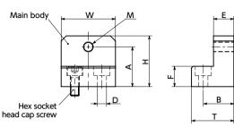
\*: Check the A dimension based on the distance from the mounting surface to the top surface of the table and select accordingly.
