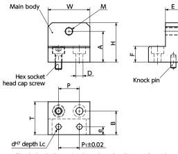
\*: Check the A dimension based on the distance from the mounting surface to the top surface of the table and select accordingly.
