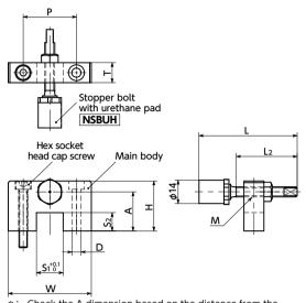
\*: Check the A dimension based on the distance from the mounting surface to the top surface of the table and select accordingly.
