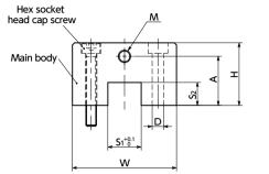
\*: Check the A dimension based on the distance from the mounting surface to the top surface of the table and select accordingly.
