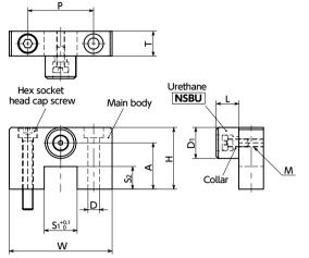
\*: Check the A dimension based on the distance from the mounting surface to the top surface of the table and select accordingly.
