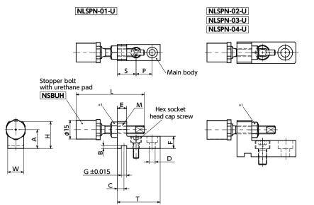
\*1: Use the lock nut on the opposite side of the side that receives the force. For NLSPN-01-U alone, in order to avoid interference with the main body, mount the lock nut on the side that receives the force.
