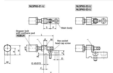
\*1: Use the lock nut on the opposite side of the side that receives the force. For NLSPNS-01-U alone, in order to avoid interference with the main body, mount the lock nut on the side that receives the force.
