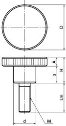
• To distinguish KNMS (SUS303) from KNML (SUS316L equivalent), **KNML** has a groove on its seating surface.
