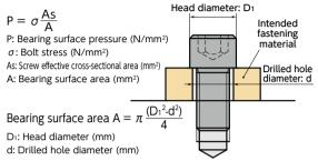
• Head Diameter and Screw Effective Cross-Sectional Area
