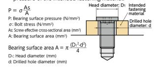
• Head Diameter and Screw Effective Cross-Sectional Area
