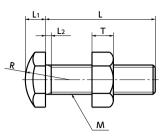
• Usage example Use the lock nut on an opposite side of the side that receives the force.
