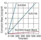
This graph compares corrosion weight loss of a test piece in 6% ferric chloride solution over
